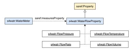
Figure 5: Water flow model
