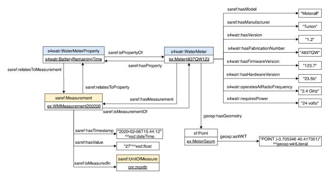
Figure 13: Example of water meter
