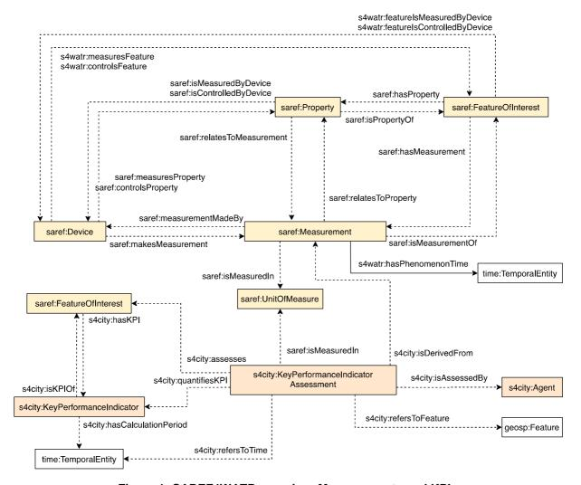
Figure 1: SAREF4WATR overview, Measurements and KPIs
