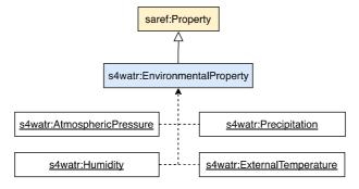
Figure 6: Environmental properties model
